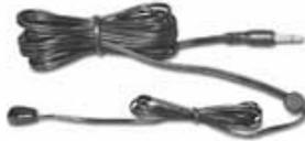
Attach IR emitter to IR window on the front of the unit for controlling an IR network system.
